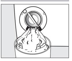
Slowly and carefully unscrew the drain filter to let the water out.
